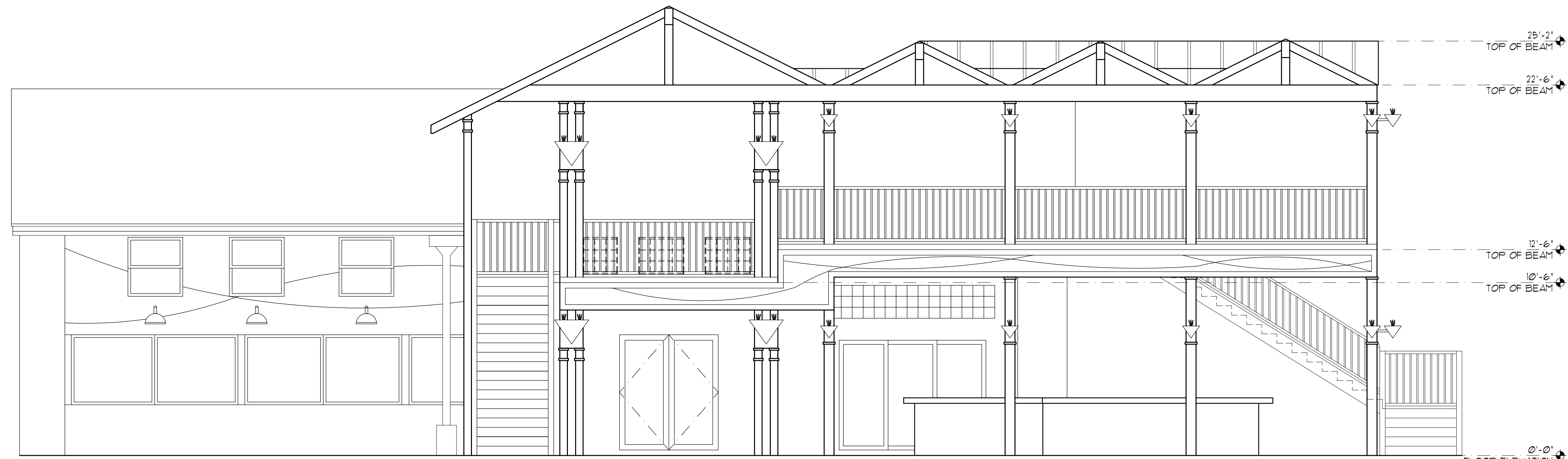
FRONT SIDE ELEVATION SCALE: 1/4" = 1'-0"
